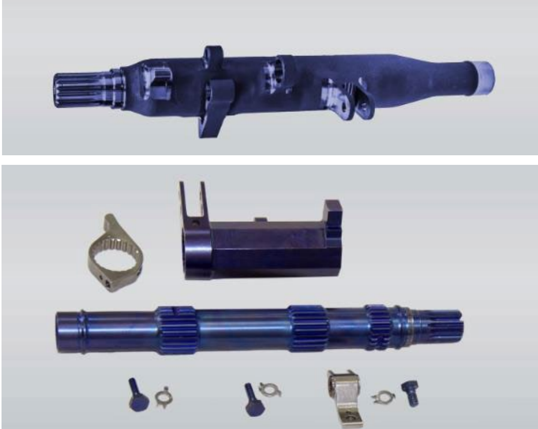
Figure 23 – Comparison of printed and conventional part, Airbus
