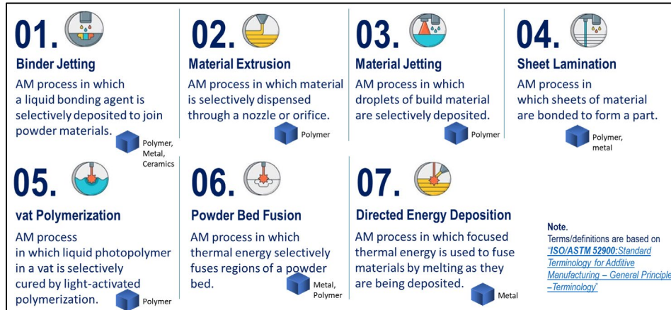
Figure 3 - Additive Manufacturing Technologies as defined in ISO/ASTM 52900
